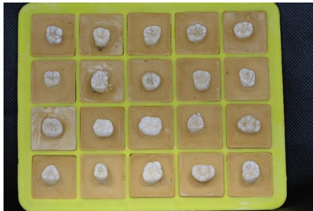
Figure 13. Teeth mounted in 25x25x25mm dental stone blocks
